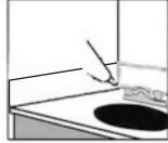
Apply "100% silicone" to the seam where the backsplash and/or sidesplash touches the granite top (indicated by grey line). Apply "kitchen & bathroom caulk" to the top edge of the splash that touches the wall.
