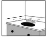
Carefully push the splash in place, making sure you firmly press it against the wall.
