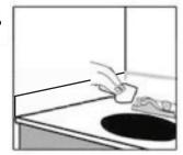
With a caulk edging tool, run it across the seams to clear away excess silicone & caulk (this technique will leave a clean line of silicone & caulk over the seams).
